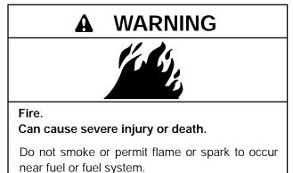
A flash fire can cause severe injury or death. Do not smoke or permit flame or spark to occur near carburetor, fuel line, fuel filter, fuel pump, or other potential sources of spilled fuel or fuel vapors. When removing fuel line or carburetor, use a proper container to catch all fuel.
